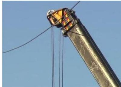
Mobile crane hits powerline – In laydown area whilst performing pick-up and carry lifts. The powerline was identified, but the layout of construction materials in the areas had changed over time. Operators were regularly reversing and traveling with boom up unloaded.
