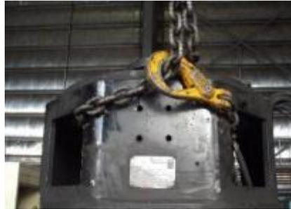
Rigging equipment failed under tension – The rigging was reeved at a high angle). This was a periodic maintenance task, not often performed by mobile maintenance personnel who only had basic rigging competency. There was a jig / cradle available to lift the component, but this was not known to the maintenance personnel.
