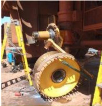
Forklift tipped, and control of load lost – The Jib used on the forklift was not fit for the weight vs length it was extended. The lift was not planned by people with an adequate level of competence to perform a heavy and complex lift.
