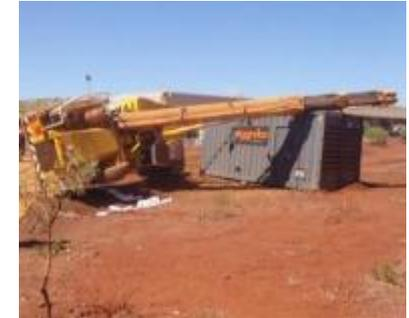
Crane rolled – Local hazard of terrain / slopes not identified because the lift, carry and placement of the load was not formally planned. The path of the crane travel was not inspected. Changes during the task introduced new hazards that were not identified and managed.
